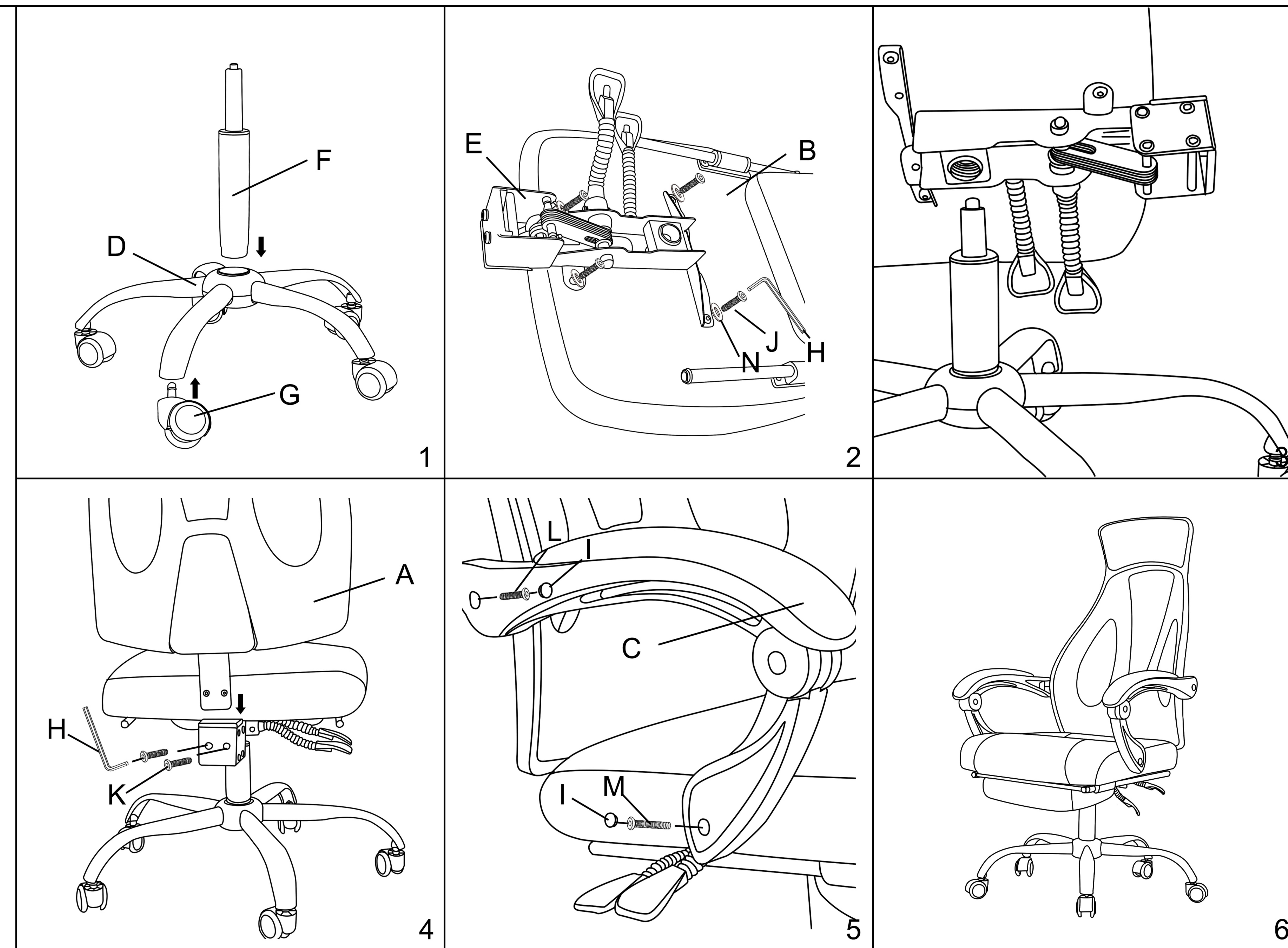
Remark: First fix screws lightly by hand and at the end of the assembly fasten the screws firmly with tools.
